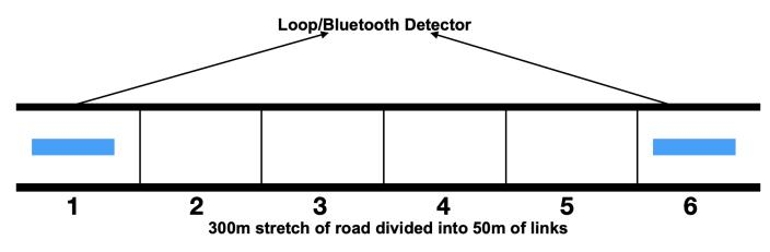
Figure 7: Road Segment Divided into Smaller Links
