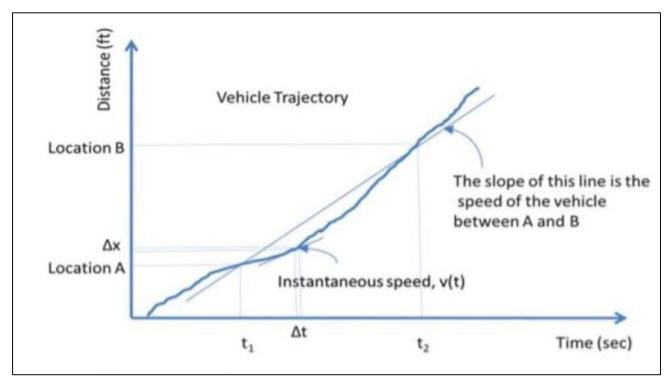
Figure 8: Trajectory of Vehicle
